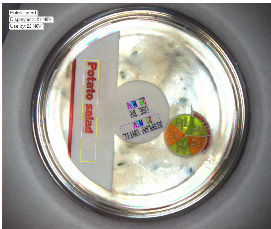
Figure 3. 2D Imaging used to verify correct labelling and 'best before' dates
