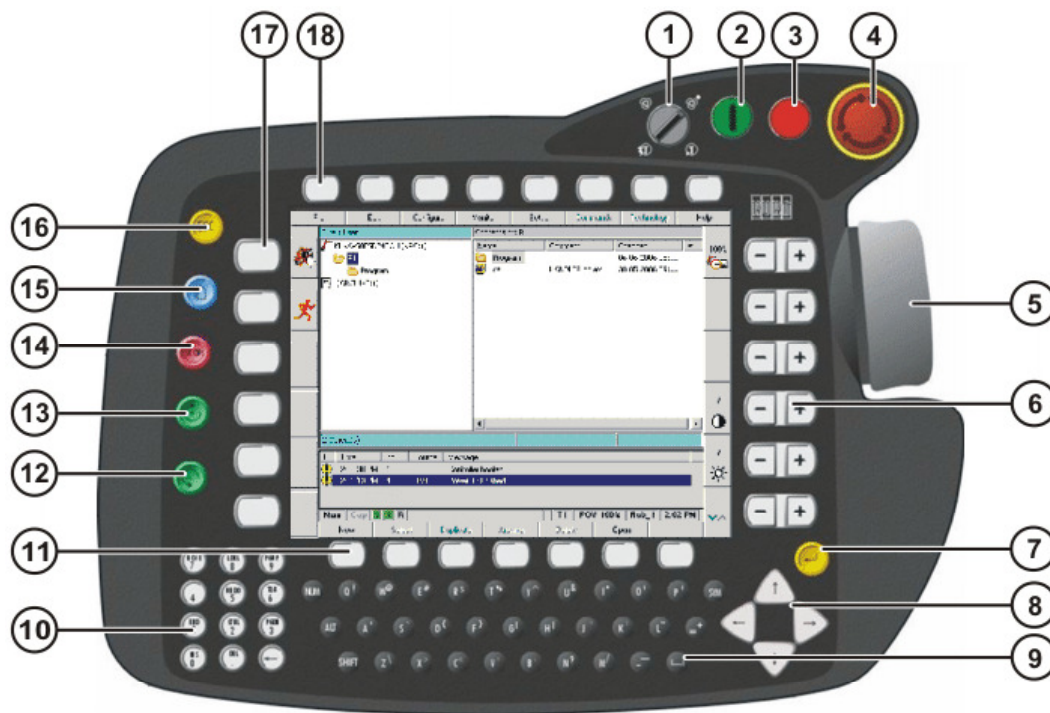
Figure 3. Teach pendant for the robot system (Source: KUKA Robots)
