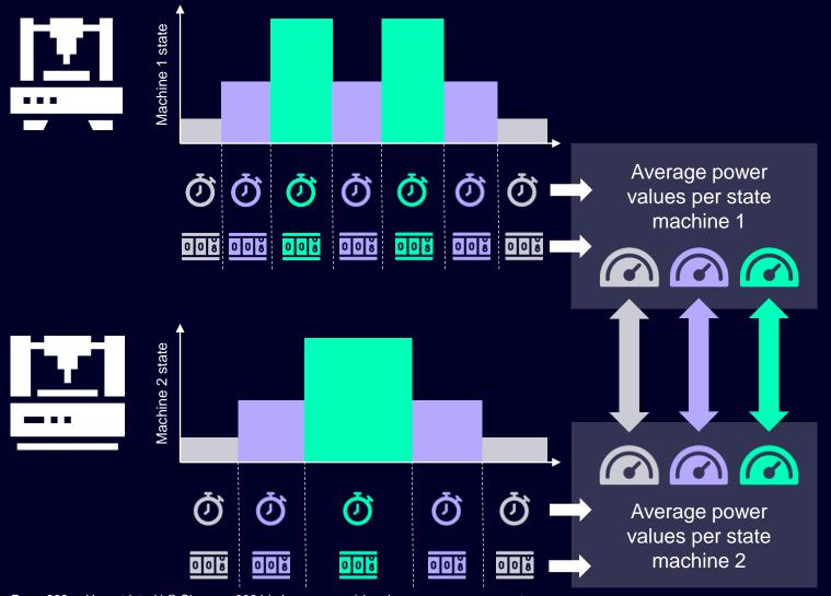
**Optime** Use cases for the EE-M – State-based energy data calculation
